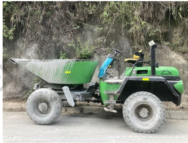
Photo 23: Tunnel spoil dump truck, losing oil
